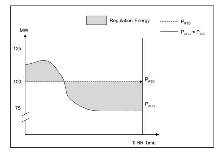
Figure 11: Error in Performance (30-Second Bandwidth not Included)
